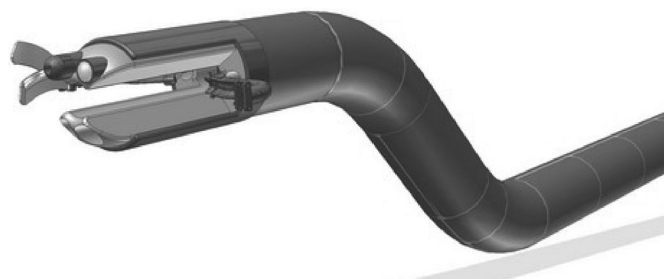
Figure 2. The Transdouglass Endoscopic Device (TED) with 2 instruments driven out.
